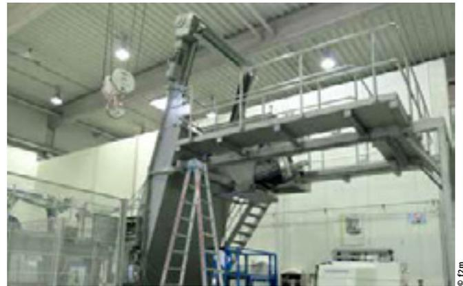
++ A bowl tipper made by DIOSNA feeds dough through a cone for further processing
