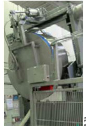
++ As soon as a bowl is in the cleaning position, a cover folds down onto the bowl and automatic cleaning starts
