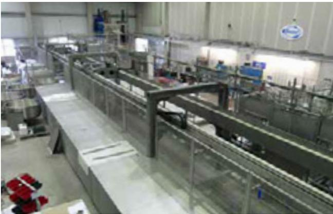
++ The transport system's structure is linear, and transport to the individual kneading and resting stations is done by two robots
